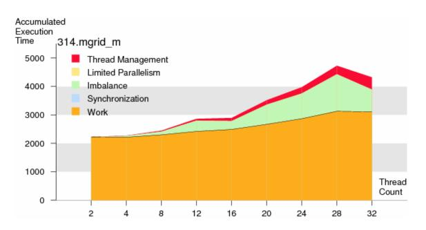
Scaling from 2 to 32 processors on an SGI Altix machine
