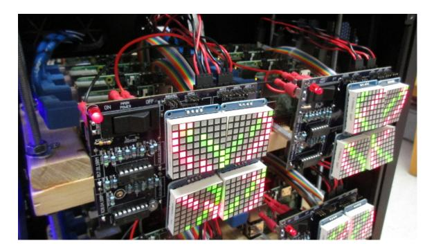
Raspberry Pi 2 Cluster, Instrumented for Detailed Power Linpack 92W, 15.4GFLOPS = 0.17 GFLOPS/W
