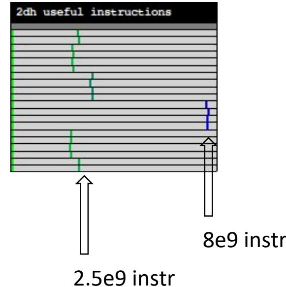
6 different processes arriving similarly after communication phase -> Then encountering load imbalance caused by instructions imbalance between the MPI processes
