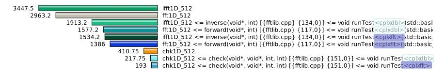
Each kernel (ifft1D\_512, fft1D\_512 and chk1D\_512) is broken down by callsite, either during the single precession or double precession step.
