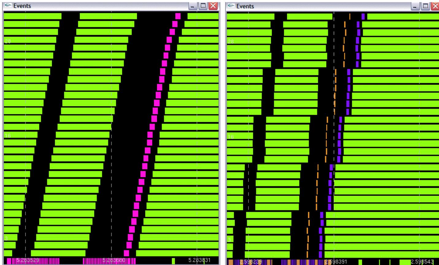
Using master to groups of workers. Time is along the x-axis and each row is a different MPI task. The master node is the bottom row
